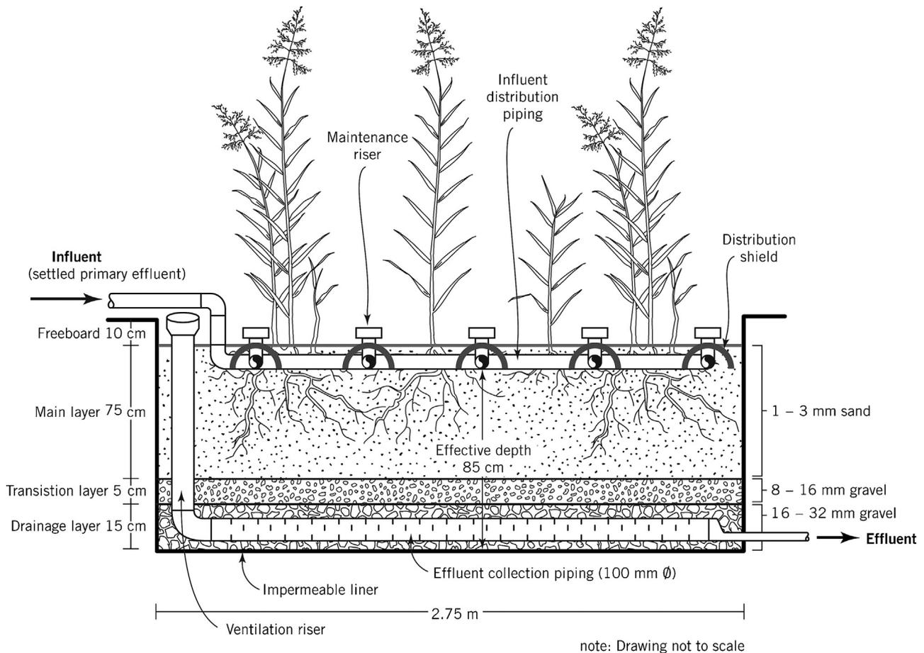
Fig. 4. Profile view of the VS design (sand-based unsaturated vertical flow systems, with and without plants: VS1, VS1p, VS2, VS2p).
