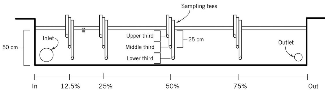
Fig. 15. Longitudinal cross-section showing location of internal sampling tees within the 50-cm deep horizontal flow beds (H50, H50p).
