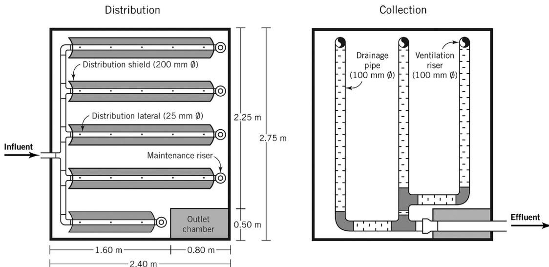
Fig. 6. Plan view of the distribution and collection systems for the vertical flow beds (VS1, VS1p, VS2, VS2p, VG, VGp, VA, VAp).
