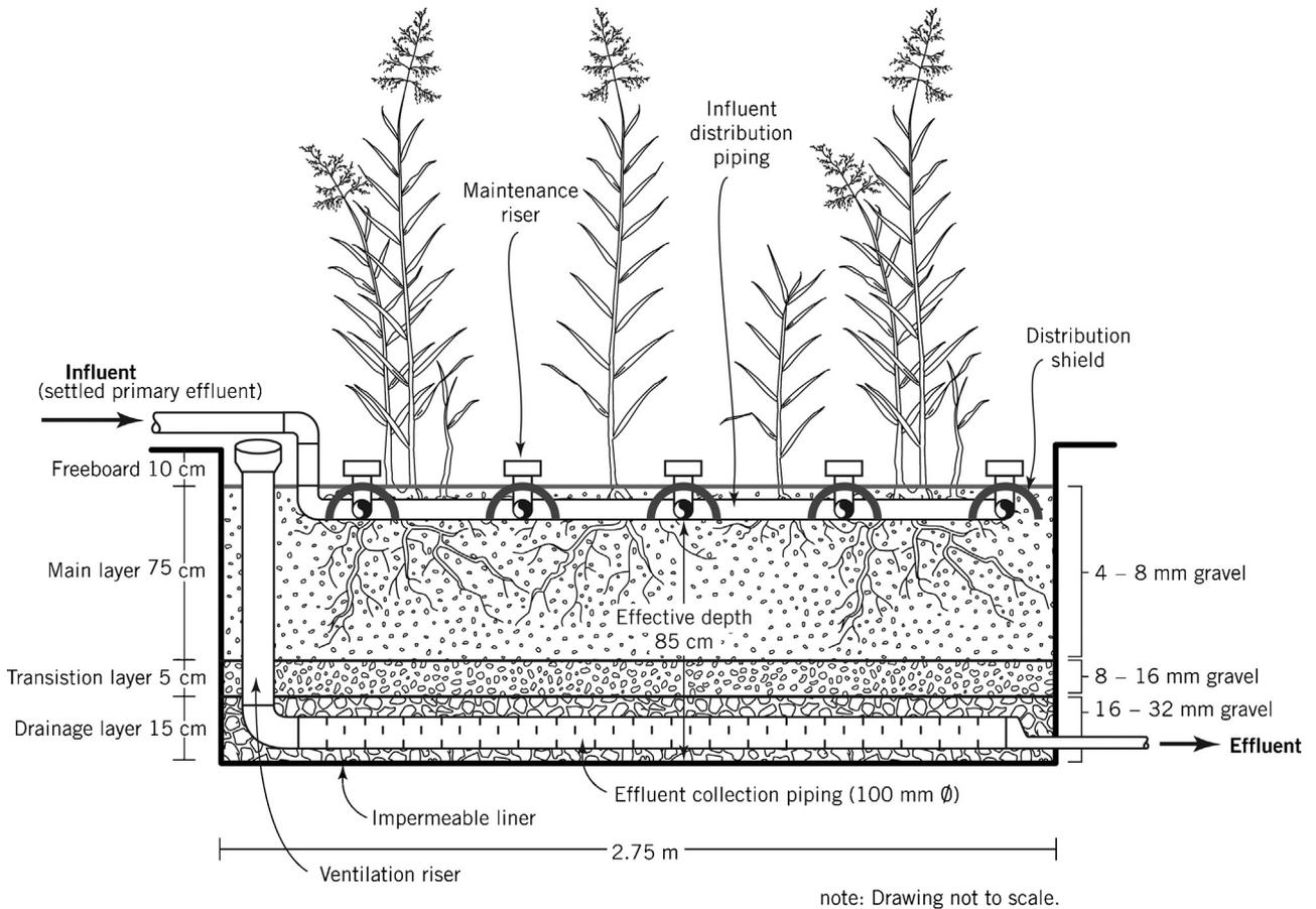
Fig. 5. Profile view of the VG design (gravel-based unsaturated vertical flow systems, with and without plants: VG, VGp).
