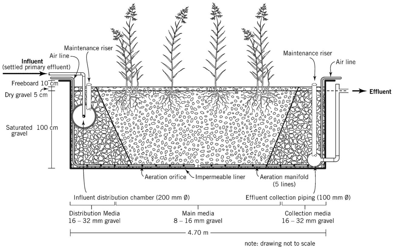
Fig. 8. Profile view of the HA design (gravel-based saturated horizontal flow systems with aeration; with and without plants: HA, HAp).
