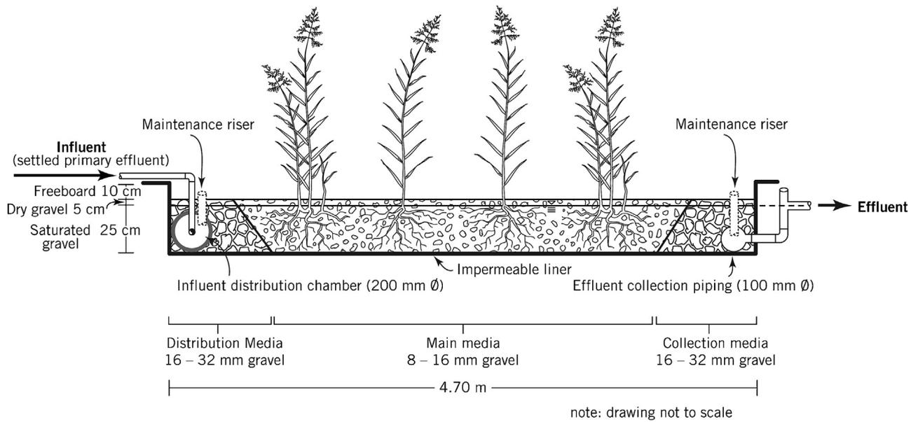
Fig. 3. Profile view of the H25 design (horizontal flow systems with a saturated depth of 25 cm).
