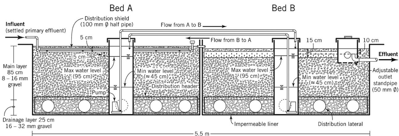
Fig. 11. Profile view of the reciprocating design (R).
