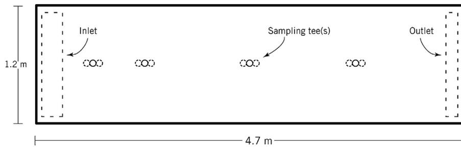
Fig. 13. Plan view of internal sampling locations for horizontal flow beds.
