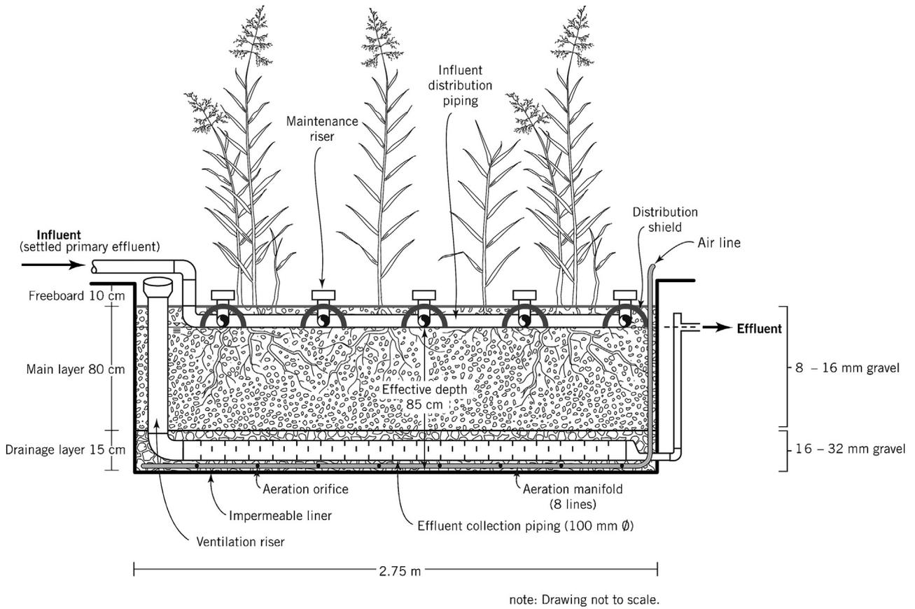
Fig. 7. Profile view of the VA design (gravel-based saturated vertical flow systems with aeration; with and without plants: VA, VAp).
