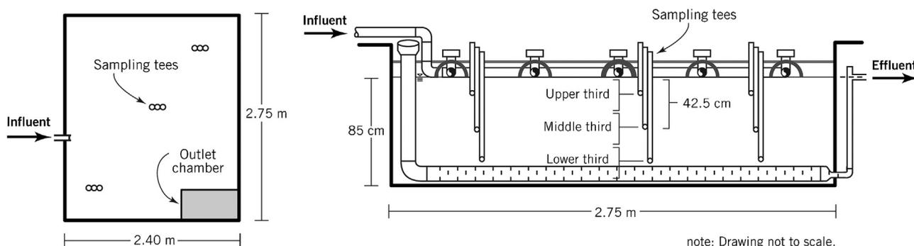
Fig. 17. Plan (left) and profile (right) views of internal sampling tees within the vertical flow beds with aeration (VA, VAp).
