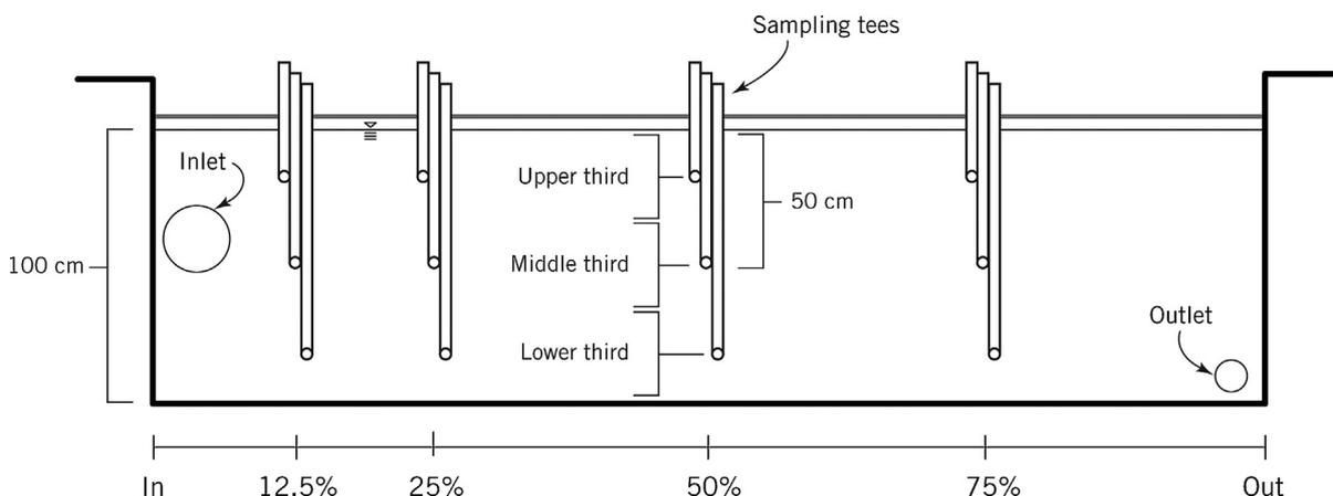
Fig. 16. Longitudinal cross-section showing location of internal sampling tees within the 100-cm deep horizontal flow beds with aeration (HA, HAp).
