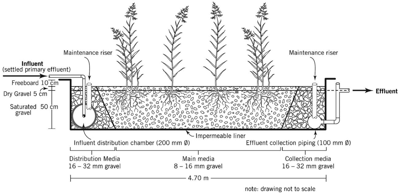
Fig. 2. Profile view of the H50 design (horizontal flow systems with a saturated depth of 50 cm).
