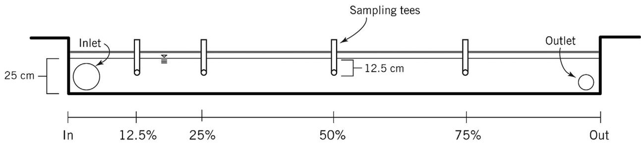
Fig. 14. Longitudinal cross-section showing location of internal sampling tees within the 25-cm deep horizontal flow beds (H25, H25p).
