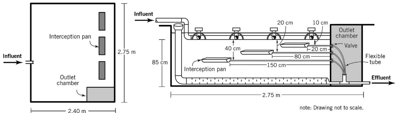
Fig. 19. Plan and profile views of interception pans in the unsaturated vertical flow beds (VS1, VS1p, VS2, VS2p, VG, and VGp).
