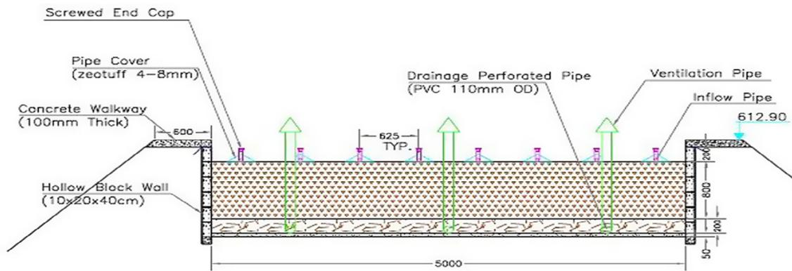
Fig. 2. Schematic diagram of the recirculating vertical flow wetland.
