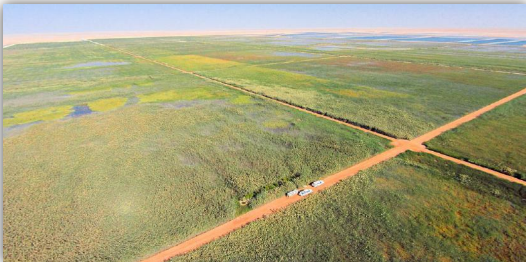
Plate 3: The 350 ha constructed wetland for which Dr Tom has been senior wetland expert for since 2011. Built in the Oman desert, each 10 ha cell was planted with a range of native wetland plants.
